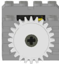
Figure 3.4: Clutch gear attached to motor
